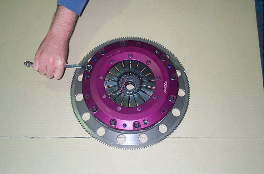
(Ref #A1) (PRESSURE PLATE COVER TO FLYWHEEL BOLTS)
