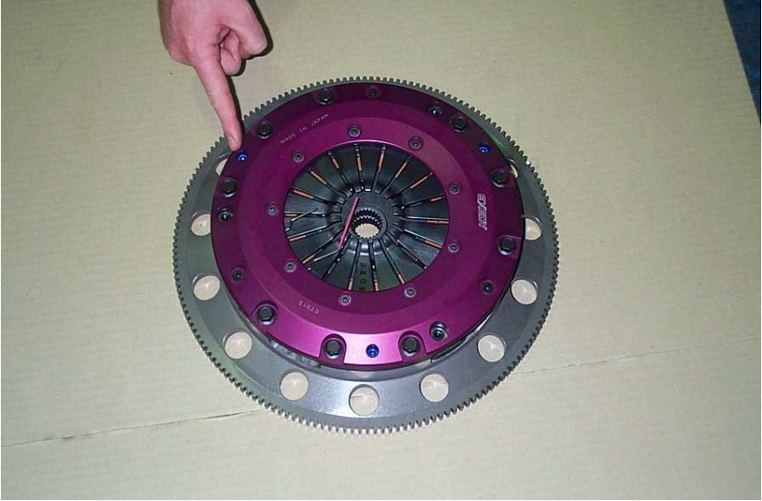
(Ref #A2) (NEVER LOOSEN THE INDICATED CAP SCREW)
